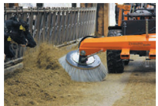
bema Groby used in a stable for sweeping up feed (PPN brush)
