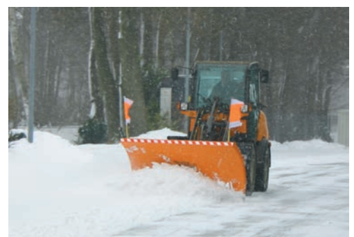
bema Snow-plough series 1100 used in winter service
