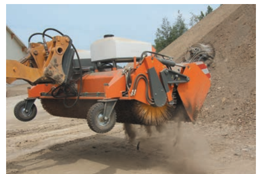
Emptying of the collection container
