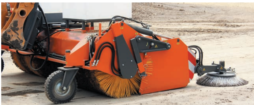
bema Titan Dual on a wheel loader with rotary side brush and water spray unit
