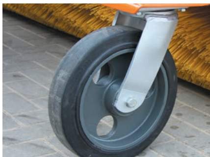
Sturdy wheels with cast wheel body Ø 360 x 85 mm
