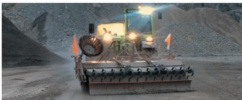
bema 75 Dual PowerMaster with bema Scraper unit and High-pressure water unit
