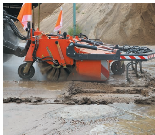
Scraping and rinsing with high-pressure
