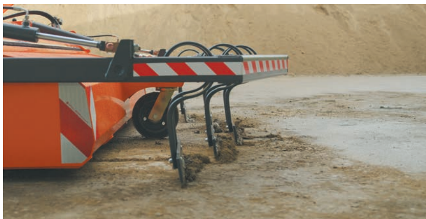
Scraper bar is divided into highly wear-resistant steel segments
