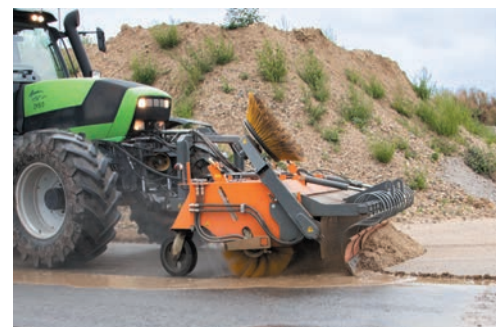
bema PowerMaster Sweeper equipped with scraper unit and rotary side brush - but without collection container.
