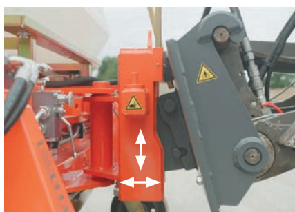
3D roller level compensation and optional swivel joint to extend the 3D equalisation
