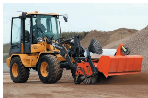
bema 35 Dual PowerMaster with water spray unit and rotary side brush (free sweeping)
