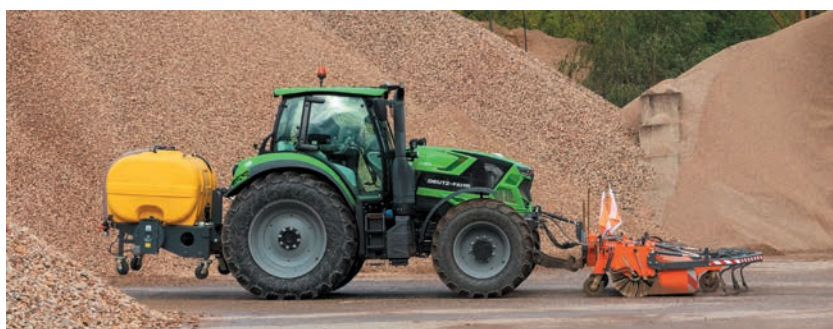
bema 35 Dual PowerMaster equipped with collection container Dual including scraper unit, high-pressure water unit, water tank in the rear and certified camera system
