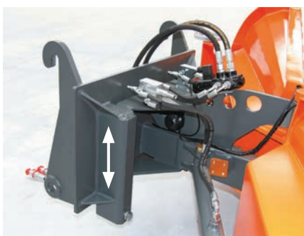
Quick change adapter, roller level compensation
