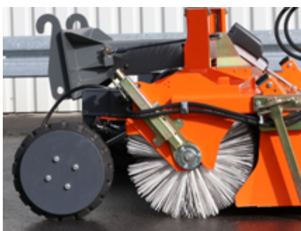
Stepless spindle adjustment of the main brush
