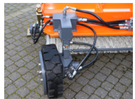
Efficient steerable wheel drive (hydraulic)
