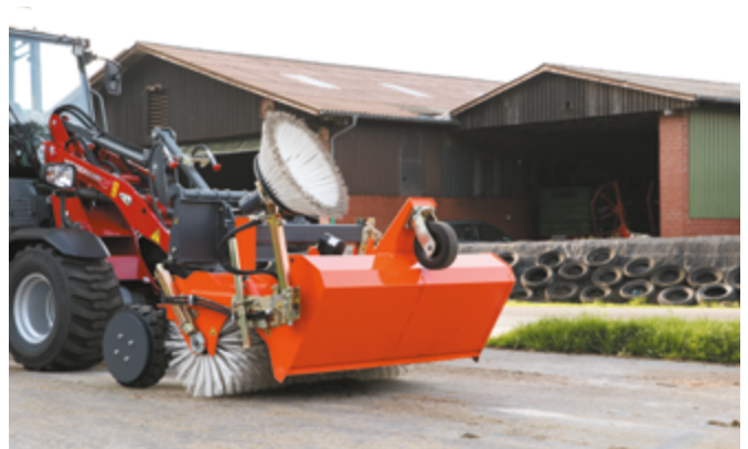
bema Sweezy® 25 Dual WD with collection container in the the proven Dual system, in this case free sweeping with an open collection container
