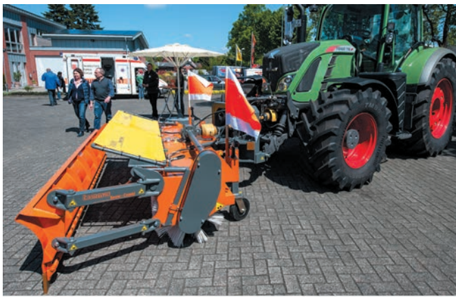
bema SnowCombi on a tractor with an optimal guard against powder snow
