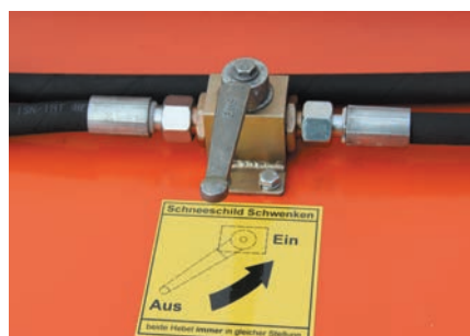
Stop valve for locking the lifted snow plough
