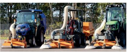
bema Suction sweeper as front mount with/without chaff blower in combination with an existing suction container or collection trailer in the rear (third-party systems)
