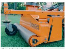
Trouble-free feed by pendulum mounted downholder roller (feed roller)
