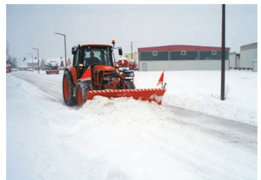
bema 700 mounted on a tractor (three-point linkage)
