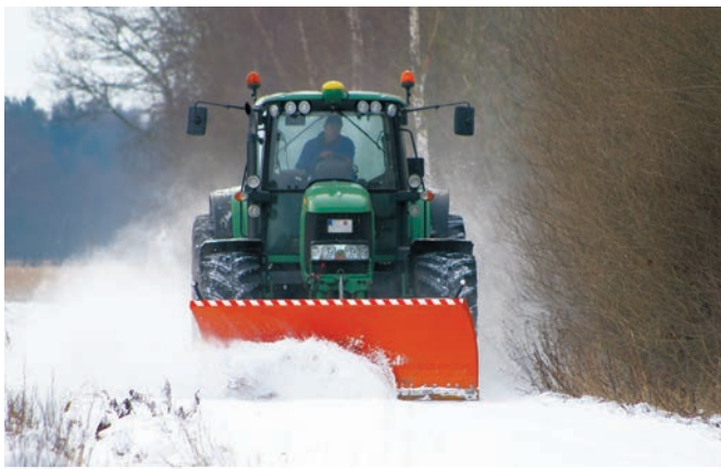
bema 1100 mounted on a tractor (front hydraulics)
