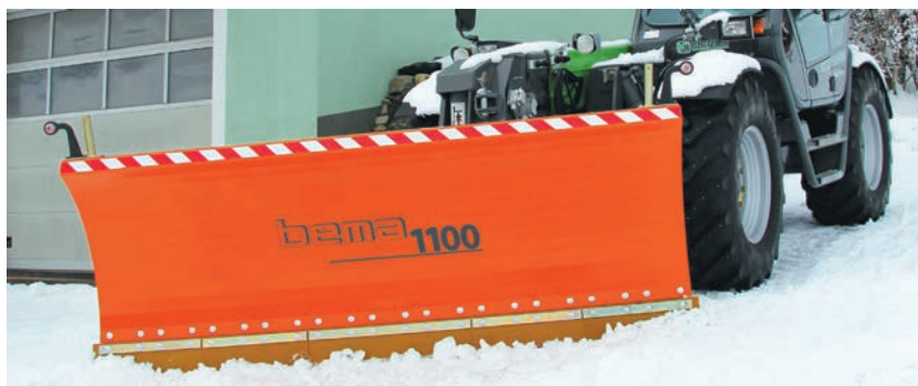
Snow plough bema 1100 with telehandler attachment (quick change adapter)
