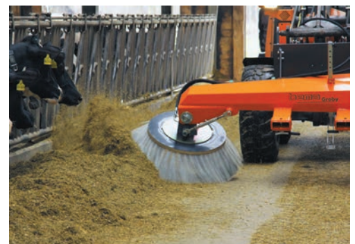
bema Groby used in a stable for sweeping up feed (PPN brush)
