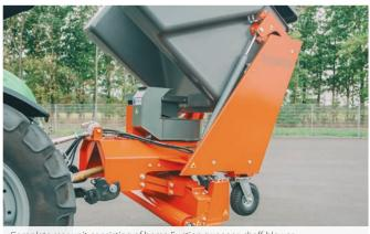
Complete rear unit consisting of bema Suction sweeper, chaff blower and bema Tipping container
