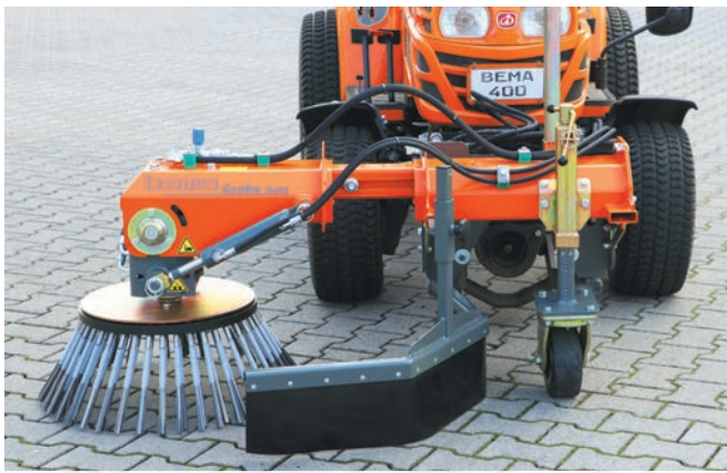
Flexible thanks to the telescopic lateral movement (300 mm)
