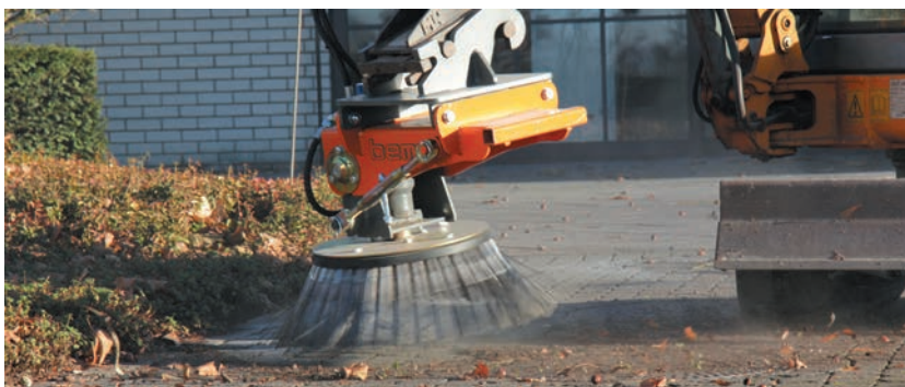
bema Groby light attached to a mini excavator
