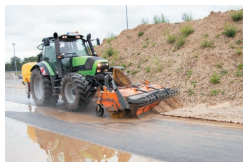
bema 75 Dual PowerMaster with scraper unit instead of collection container
