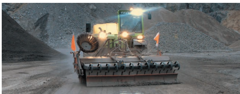
bema 75 Dual PowerMaster with scraper unit instead of collection container, rotary side brush, high pressure water unit and water tank in the rear
