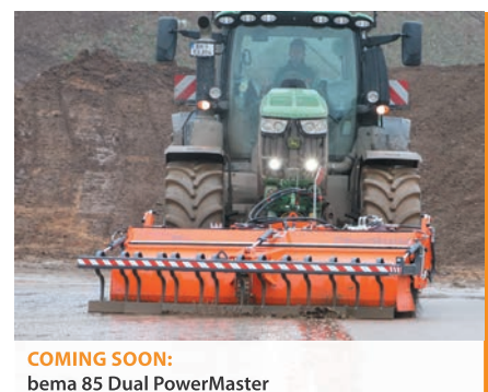
3D roller level compensation and optional swivel joint to extend the 3D equalisation
